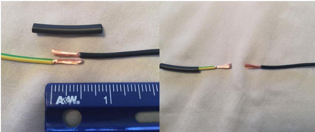
**Cut a piece of shrink tube and slide it onto one of the wires (If you are using electrical tape to cover your joint, skip this step).** If you are using shrink tube to cover your connection, you will want to slide the shrink tube onto the wire before connecting the wires. The piece of shrink tube should be longer than the area being soldered.
